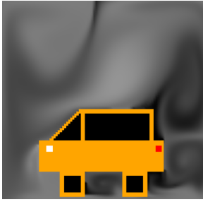
Fig. 20: A car model made from solid objects. Note that smoke does not pass through the car
